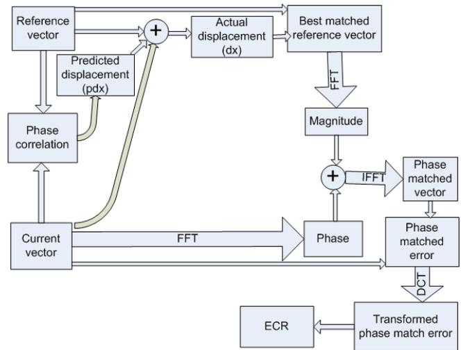
Fig. 3. Block diagram of energy concentration ratio generation.
